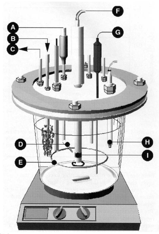
A. Reference Electrode B. Inlet C. Outlet D. Luggin Capillary E. Counter Electrode F. Rotating Cylinder G. Temperature Probe H. pH Electrode
